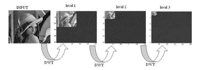
**DESCRIPTION:** The **PROPOSED DESIGN** is a flexible hardware architecture of multilevel decomposition Discrete Wavelet Transform (DWT) for image compression applications to eliminate redundant information from the transmitted images or video frames over the wireless channel. It facilitates to images of size 64×64, 128×128, 256×256, and 512× 512 pixels and capable of seven levels of decomposition. In the **MODIFICATION** we perform process to improve **PSNR** ratio.
